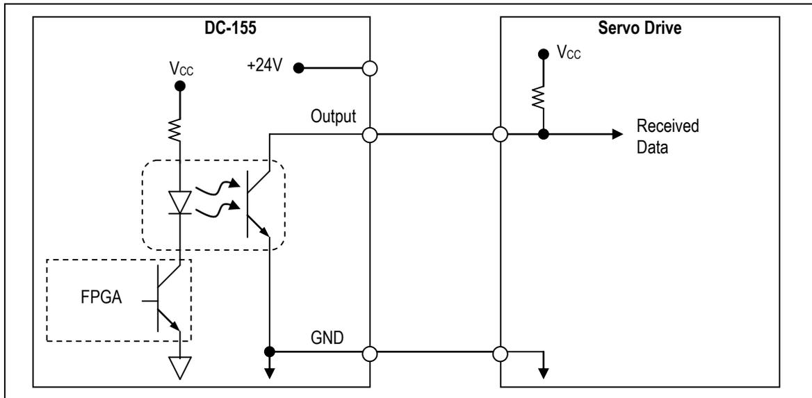
**Figure 8-6: Wiring Example of a Servo-Related Output in Which the Servo Drive Does Not Use an Opto-Isolator**
