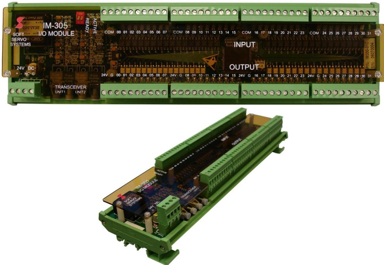
**Figure 3-1: Photos of the IM-305 General I/O Module**
