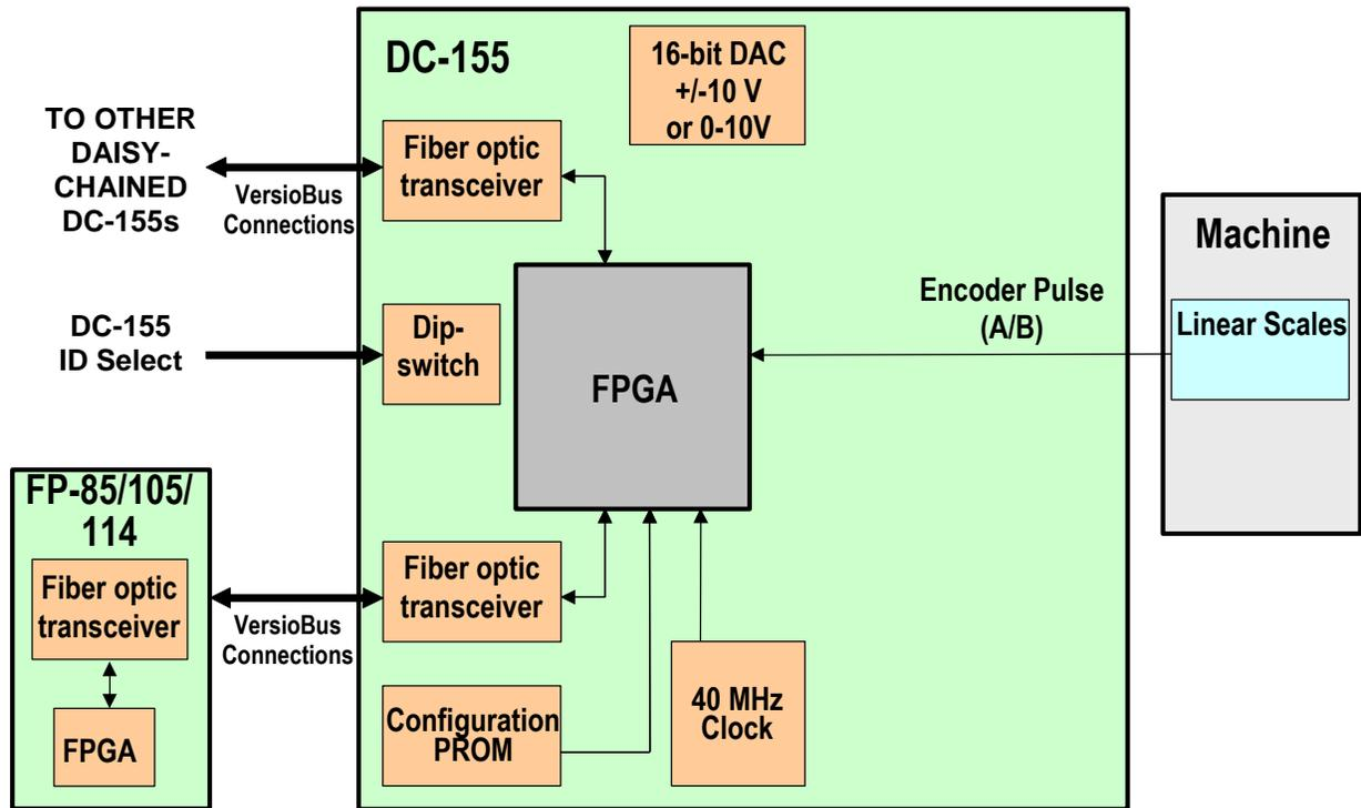
**Figure 2-17: Schematic Diagram: DC-155 FPGA Hardware Shell Architecture for Linear Scales**
