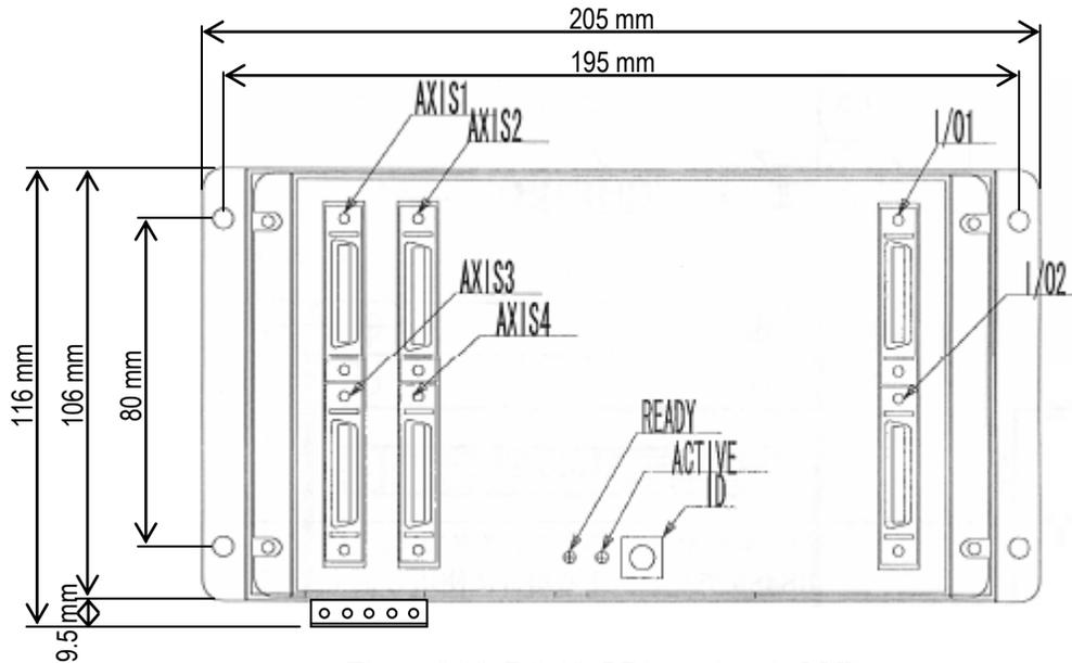
Figure 2-18: DC-125J Dimensions in Millimeters
