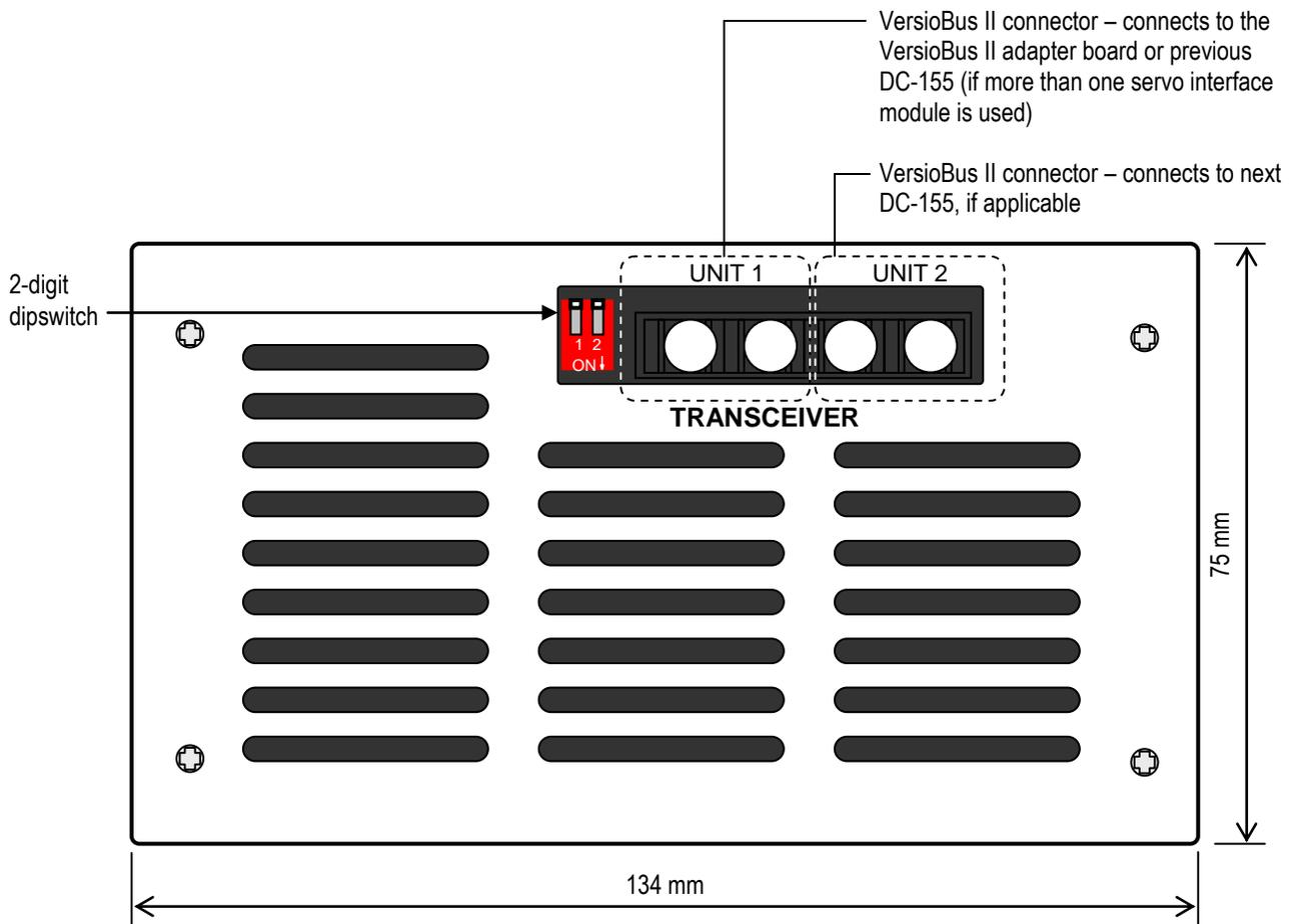
**Figure 2-3: DC-155 VersioBus II Remote Servo Interface Schematic Bottom Diagram**
