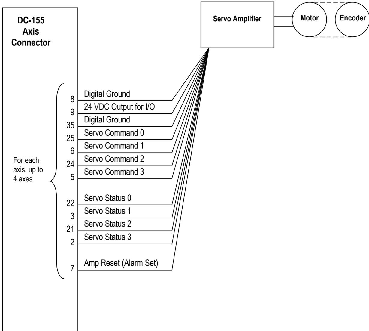
**Figure 2-13: Wiring Diagram for Optional Servo Motor Connections**
