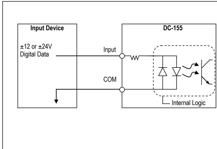
**Figure 8-3: Bi-Directional Signal Example #1**
