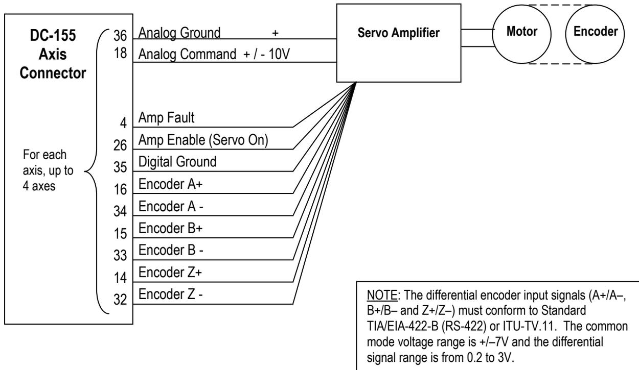
**Figure 2-11: Wiring Diagram for Essential Servo Motor Connections in the VersioBus II System When the Servo Amplifier Provides the Encoder Signals**
