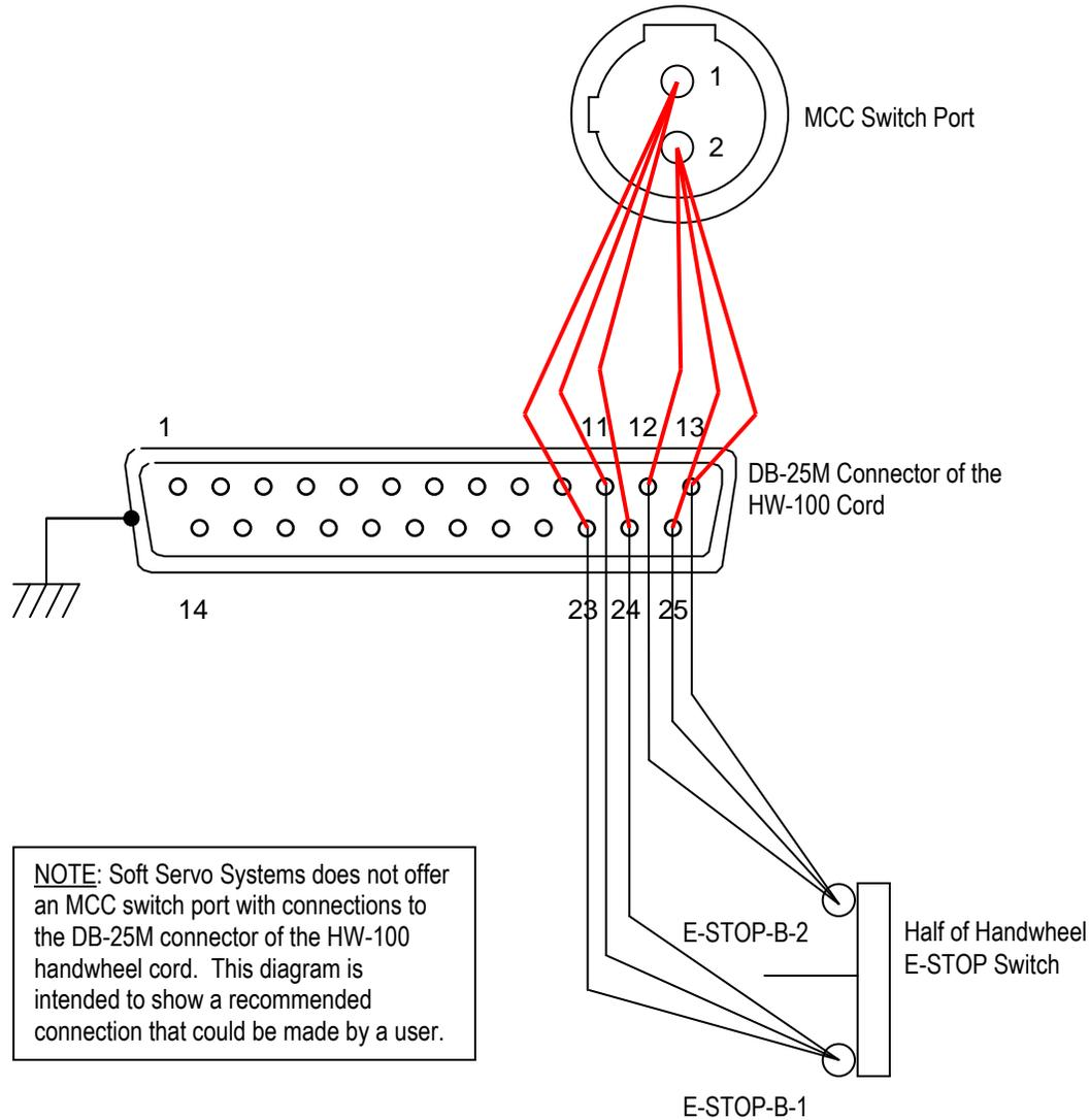
**Figure 6-4: Wiring Diagram for E-STOP/Handwheel Connection**
