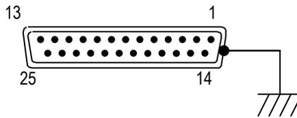
Female 25-Pin DB Connector On the Ribbon Cable for Connection to the J1 Header Block on the FP-85, the J1 Header Block on the FP-105 or the J1 Header Block on the FP-114
