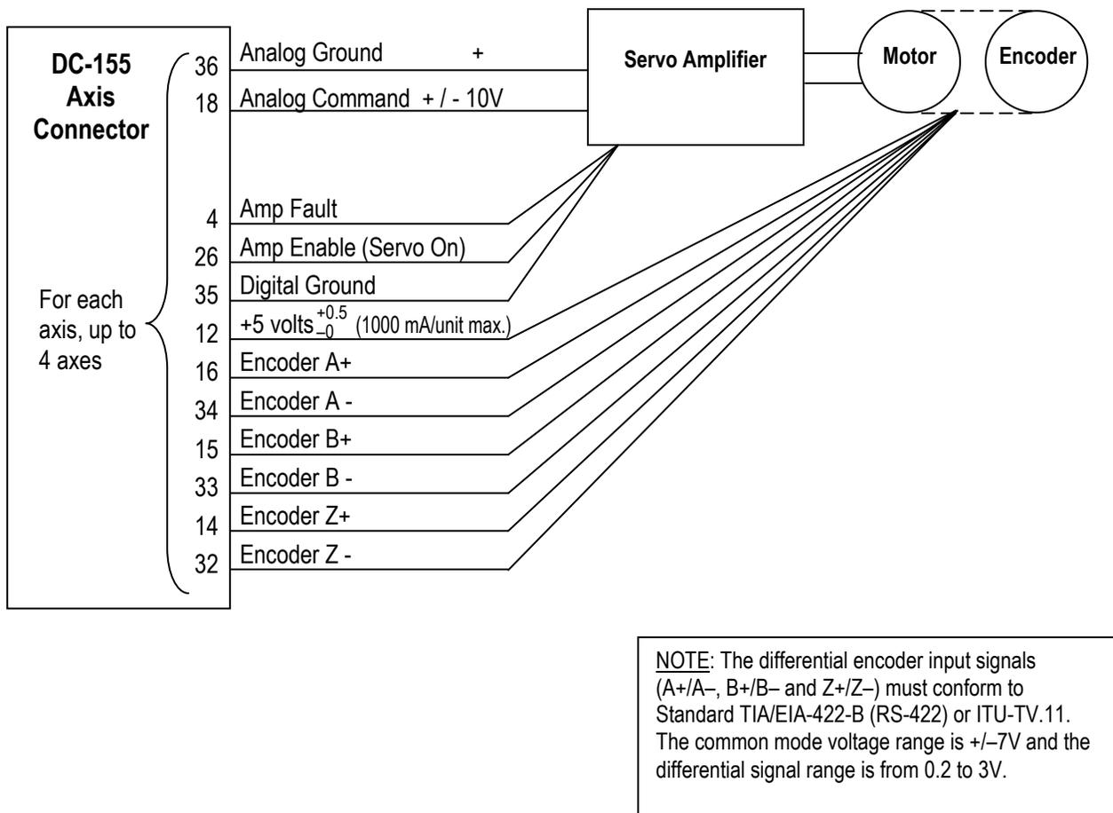
**Figure 2-12: Wiring Diagram for Essential Servo Motor Connections in the VersioBus II System When the Signals Come Directly From the Encoder**
