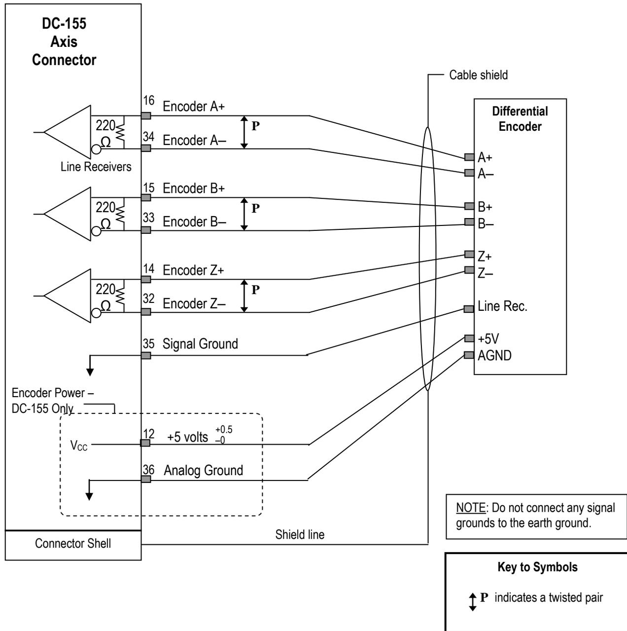
**Figure 2-14: Wiring Diagram for a Typical Connection Between a Differential Encoder and the DC-155**
