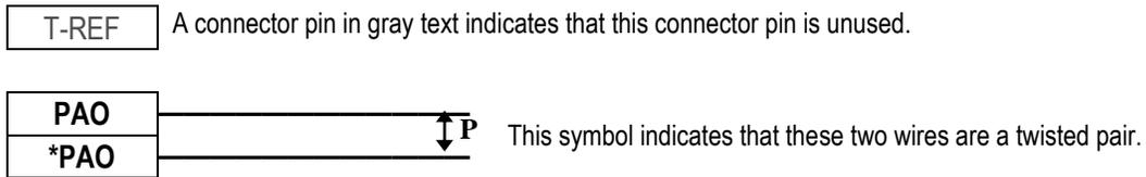
**Figure 2-15: Key to Recommended Direct Cable Connections Tables**
