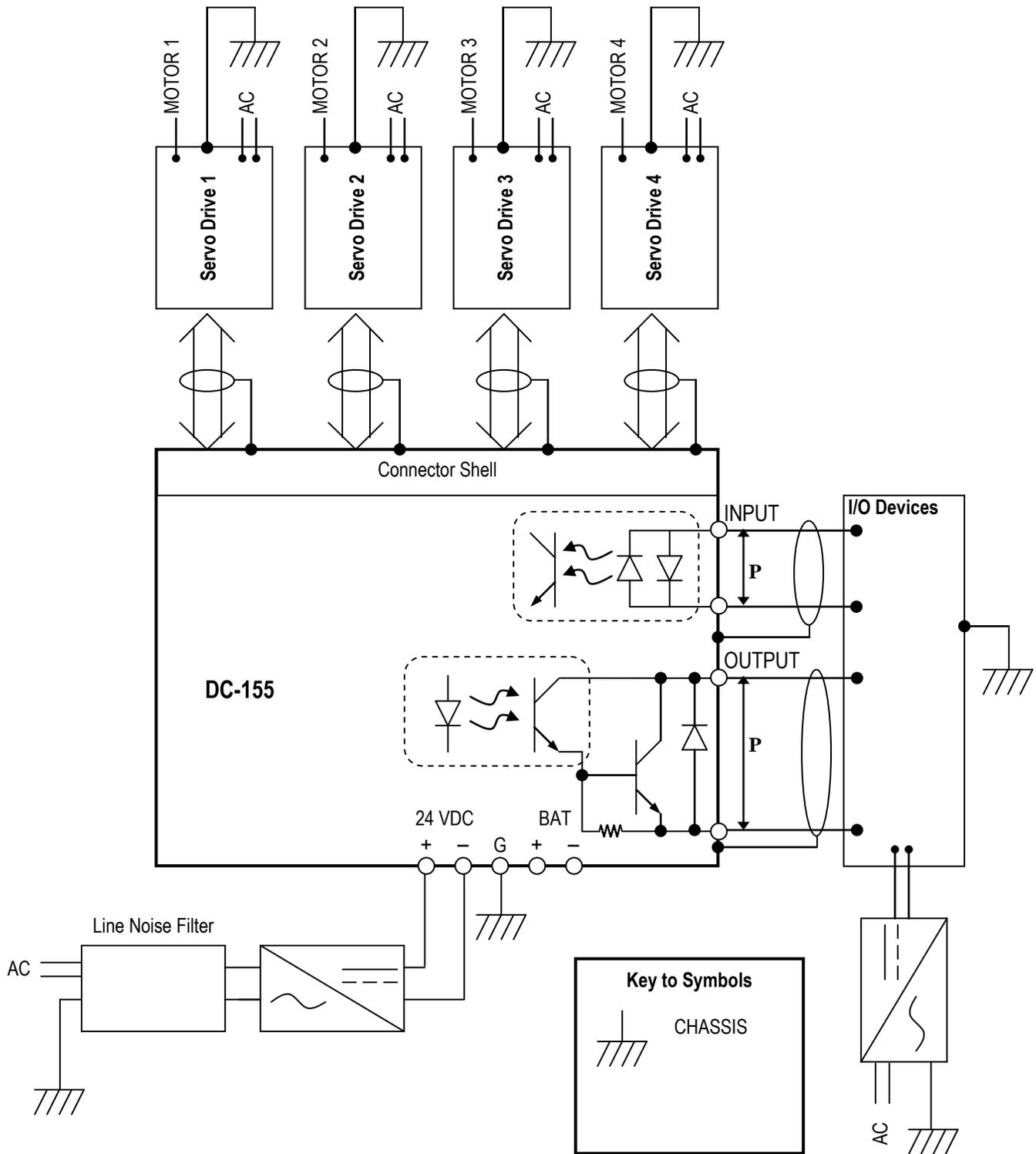
**Figure 8-13: Wiring Example of a Ground Connection for a DC-155**
