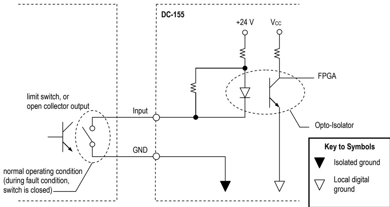
**Figure 2-7: Internal Circuitry and Wiring Diagram for DC-155 Servo-Related Digital Inputs**
