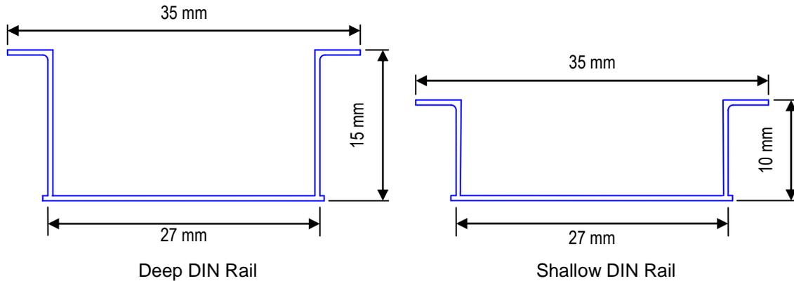
**Figure 7-1: DIN Rail Dimensions**
