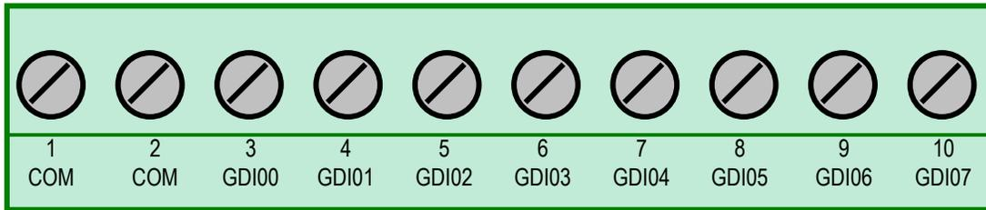
**Figure 3-5: Screw Terminal Numbers for General Digital Inputs (TERMINAL BLOCK 1 – IM-305)**
