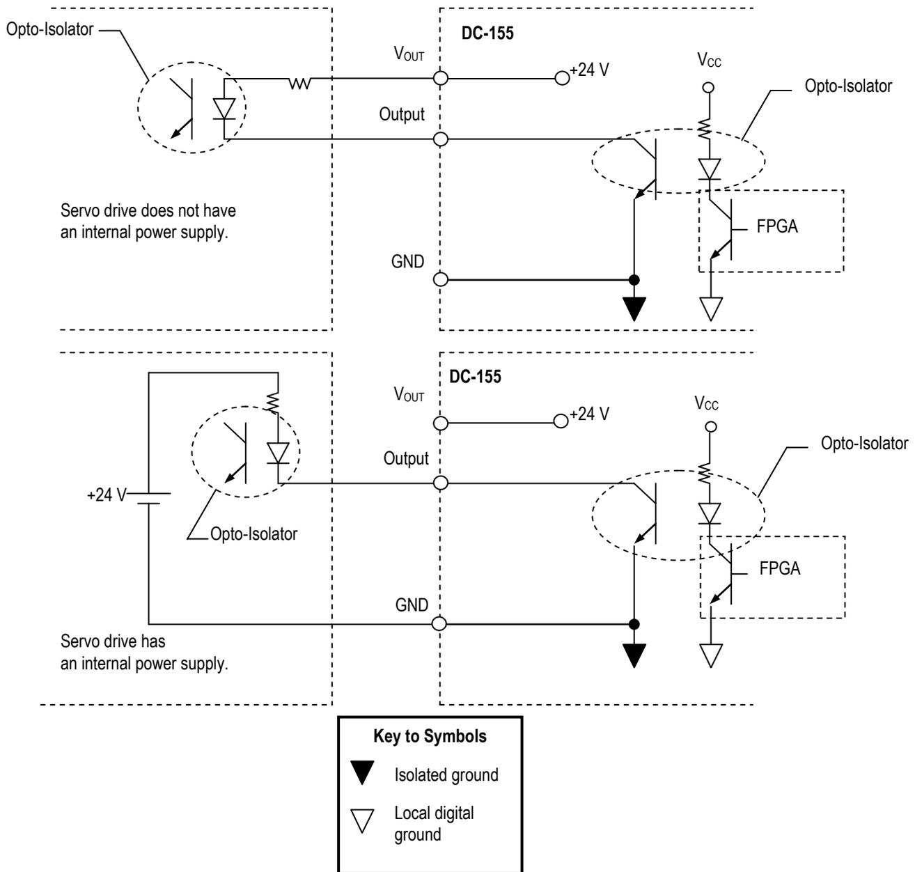
**Figure 2-8: Internal Circuitry and Wiring Diagram for DC-155 Servo-Related Digital Outputs**
