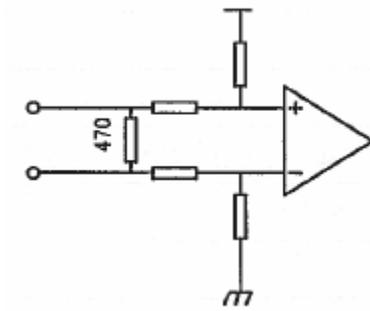
**Figure 2-23: Internal Circuitry and Wiring Diagram for DC-125J IN3 Inputs**
