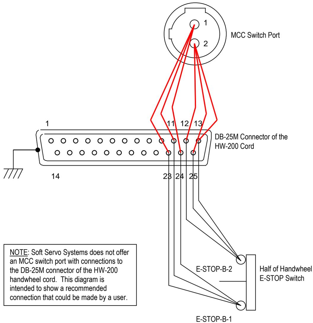
**Figure 5-4: Wiring Diagram for E-STOP/Handwheel Connection**
