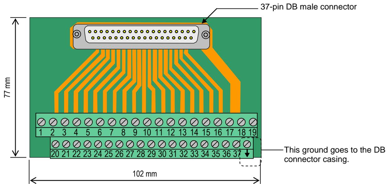
**Figure 4-8: TB37BD Breakout Box Terminal Number Assignments**
