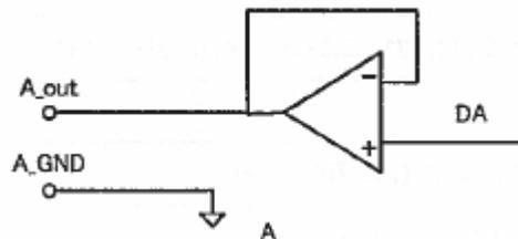
**Figure 2-19: Internal Circuitry and Wiring Diagram for DC-125J OUT4 Outputs**
