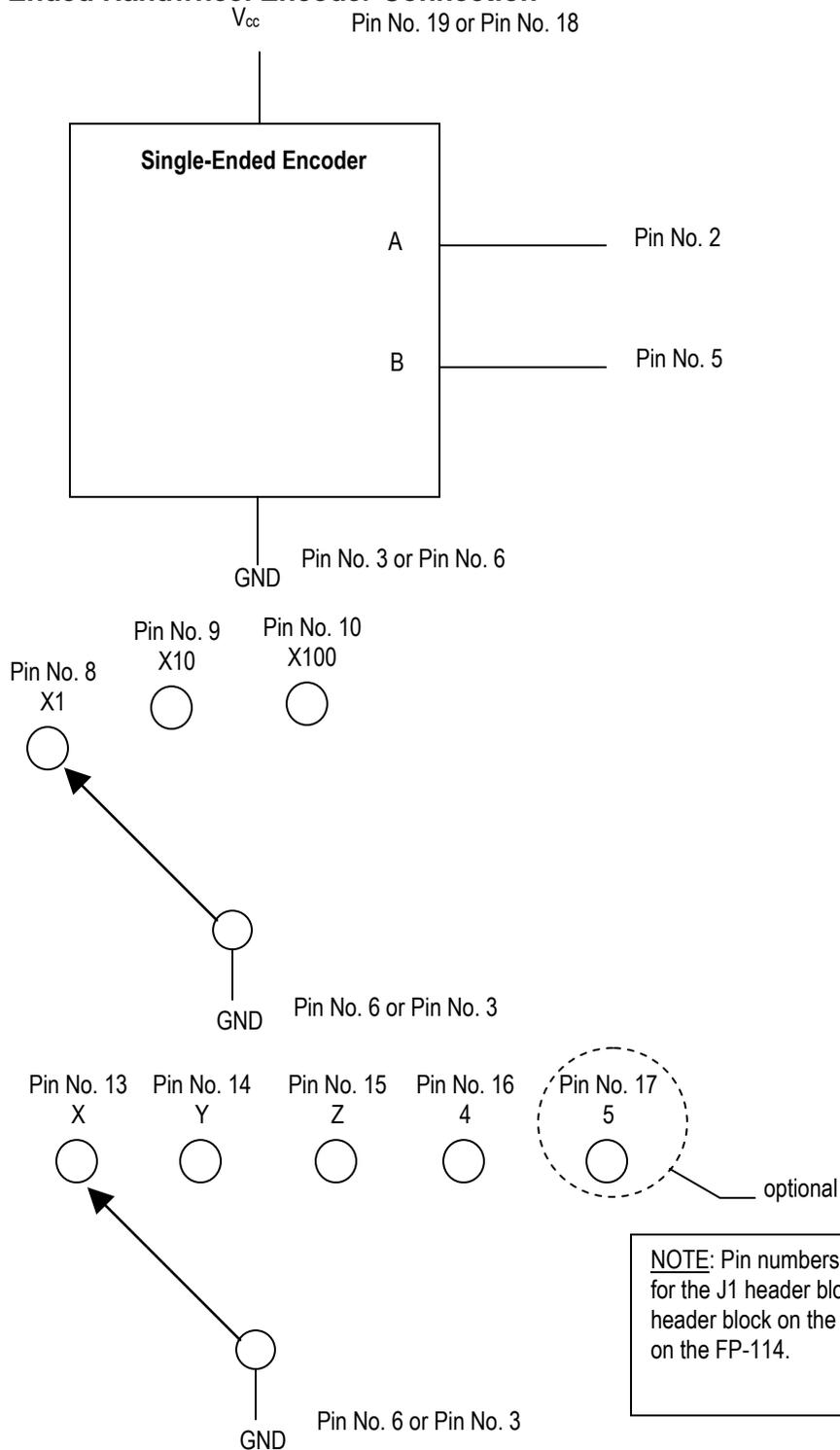
**Figure 1-7: Internal Circuitry and Wiring for a Single-Ended Handwheel Encoder Connection**
