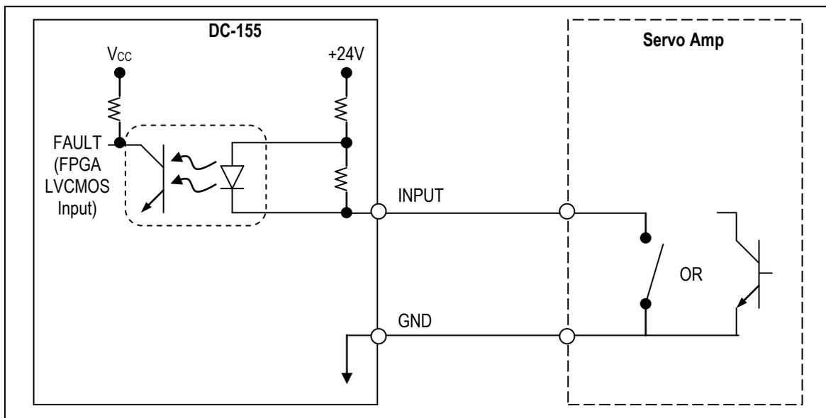
**Figure 8-9: Wiring Example of a Pull-Down Switch or Open Collector Logic Signal**
