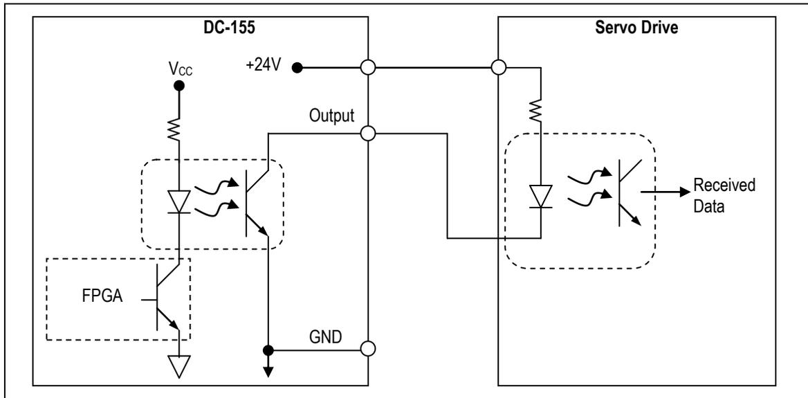
**Figure 8-4: Wiring Example of a Servo-Related Output in Which the Servo Drive Uses Power Provided by the DC-155 to Operate the Opto-Isolator**
