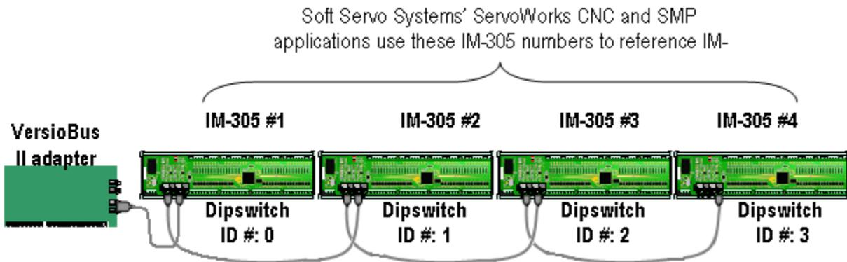
**Figure 3-2: Dipswitch ID Numbers for Daisy-Chained IM-305s**
