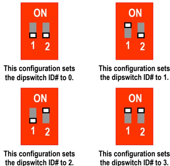
**Figure 3-3: Possible 2-Digit Dipswitch Configurations**
