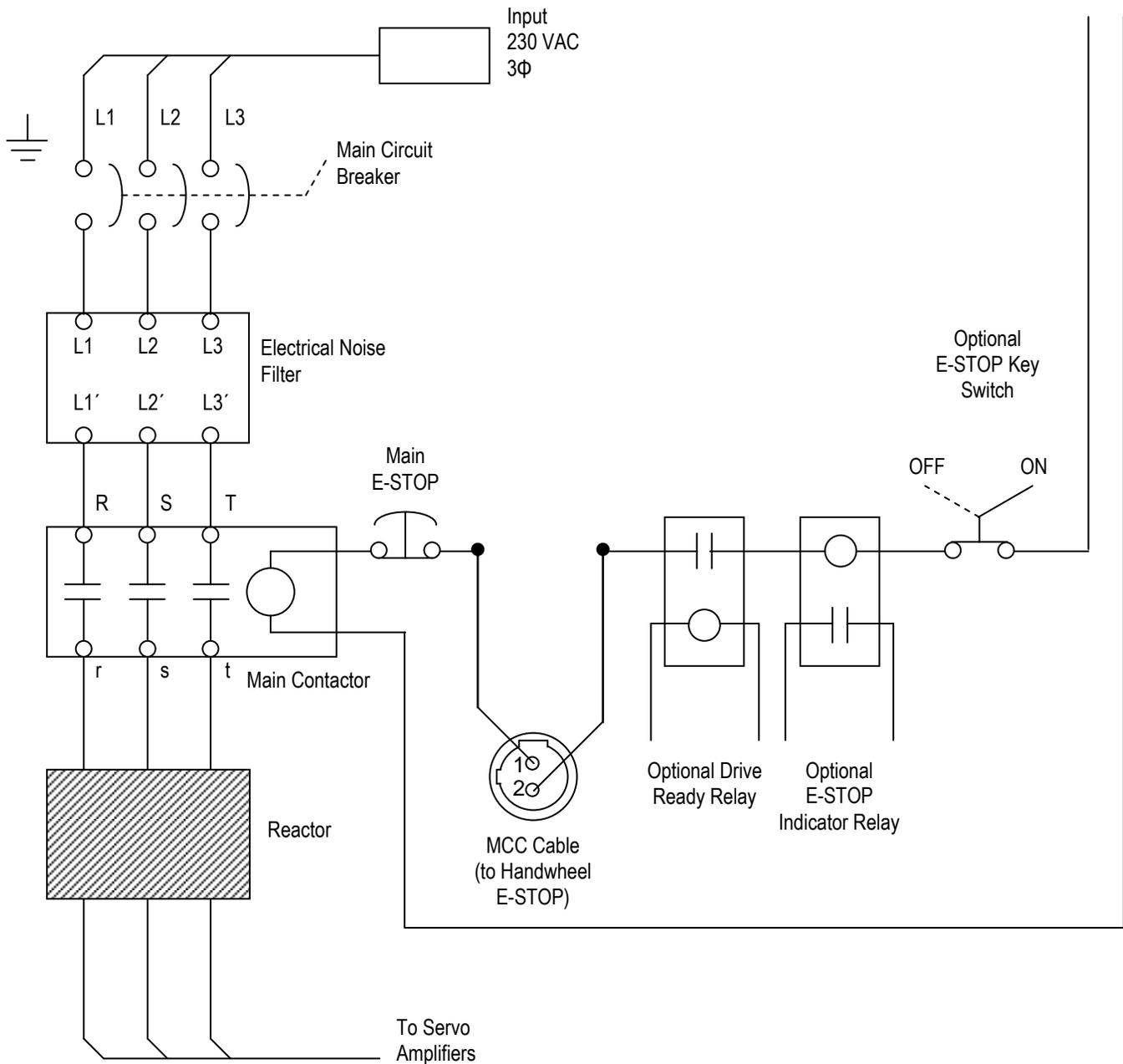
**Figure 8-1: Typical Power Wiring Diagram**
