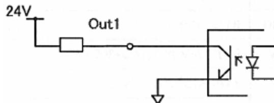
Figure 2-20: Internal Circuitry and Wiring Diagram for DC-125J OUT1 Outputs
