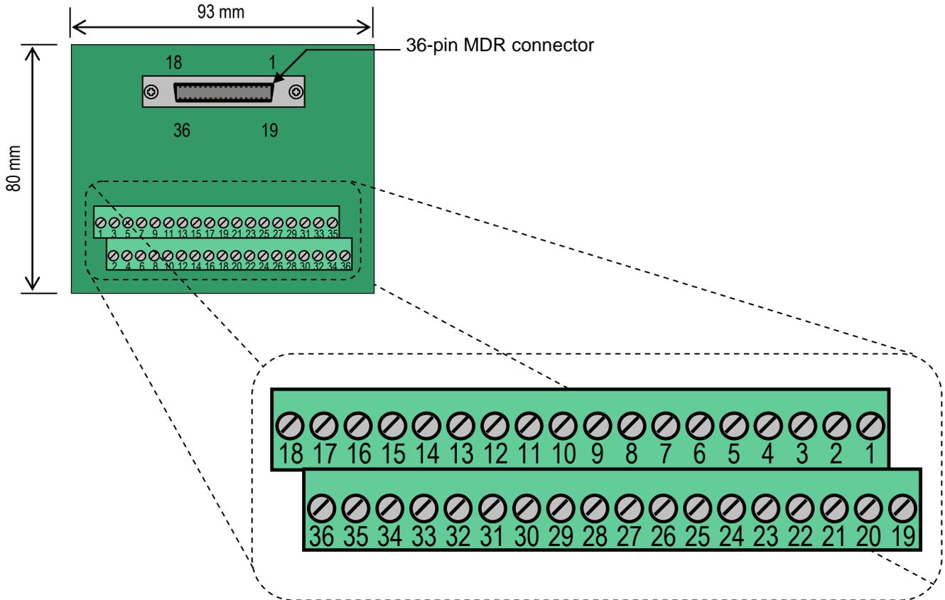
**Figure 4-6: TB36B Breakout Box Terminal Number Assignments**
