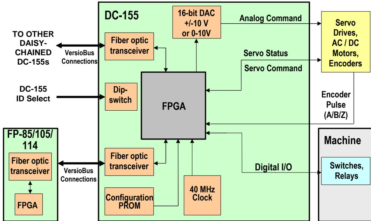
Figure 2-16: Schematic Diagram: DC-155 FPGA Hardware Shell Architecture for AC and DC Motors
