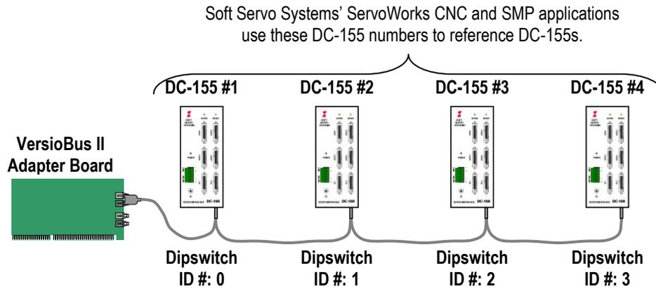
**Figure 2-5: Dipswitch ID Numbers for Daisy-Chained DC-155s**
