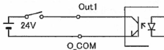
**Figure 2-22: Internal Circuitry and Wiring Diagram for DC-125J OUT2 Outputs**
