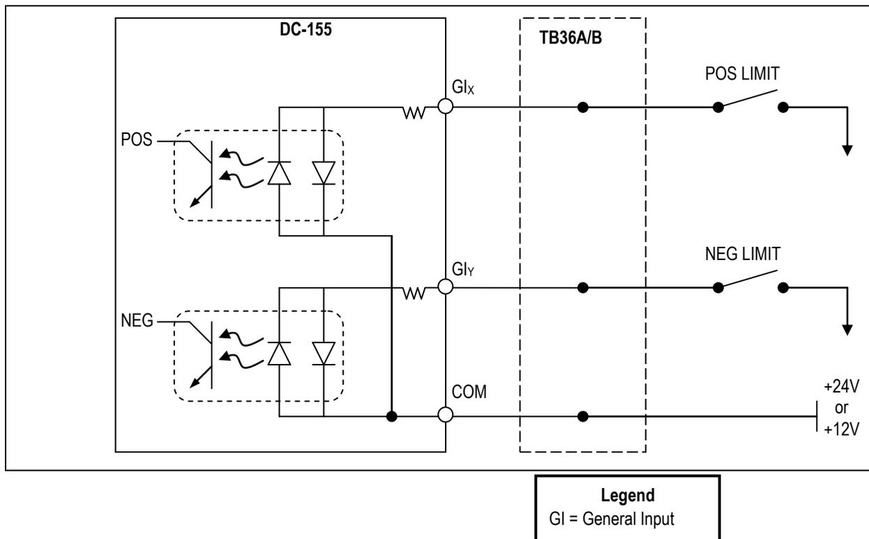
**Figure 8-11: Wiring Example of Normally Closed Limit Switches (Common “+” Supply Connection) Connected to DC-155 General Input**
