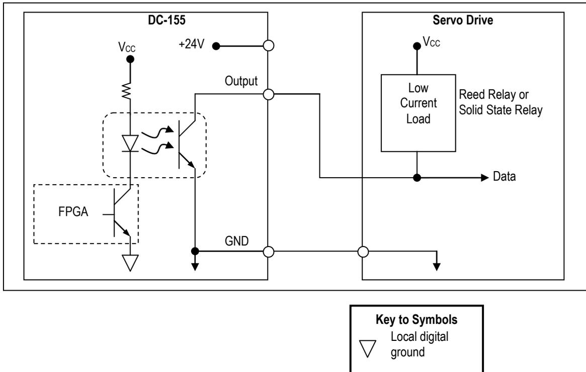
**Figure 8-8: Wiring Example of a Servo-Related Output in Which the Servo Drive Employs DC-155 Output to Drive Low Current Load Without the +24V Provided**
