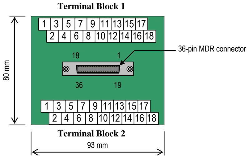
**Figure 4-2: TB36A Breakout Box Terminal Number Assignments**
