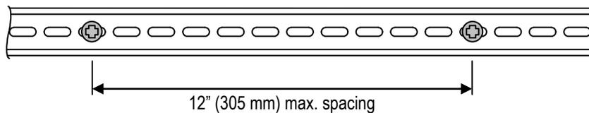
**Figure 7-2: DIN Rail Mounting**
