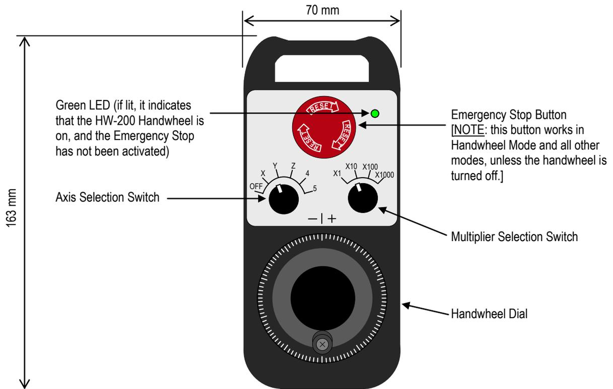
**Figure 5-2: HW-200 Handwheel Schematic Diagram**
