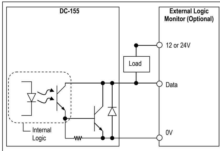
**Figure 8-12: Wiring Example of a General Digital Output Signal for a DC-155**
