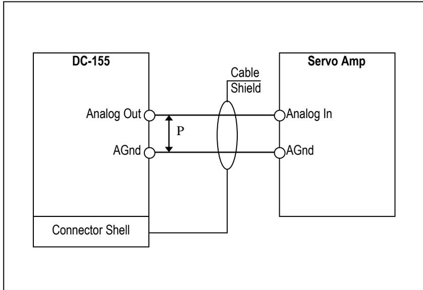
**Figure 8-2: Wiring Example of an Analog Output Signal**
