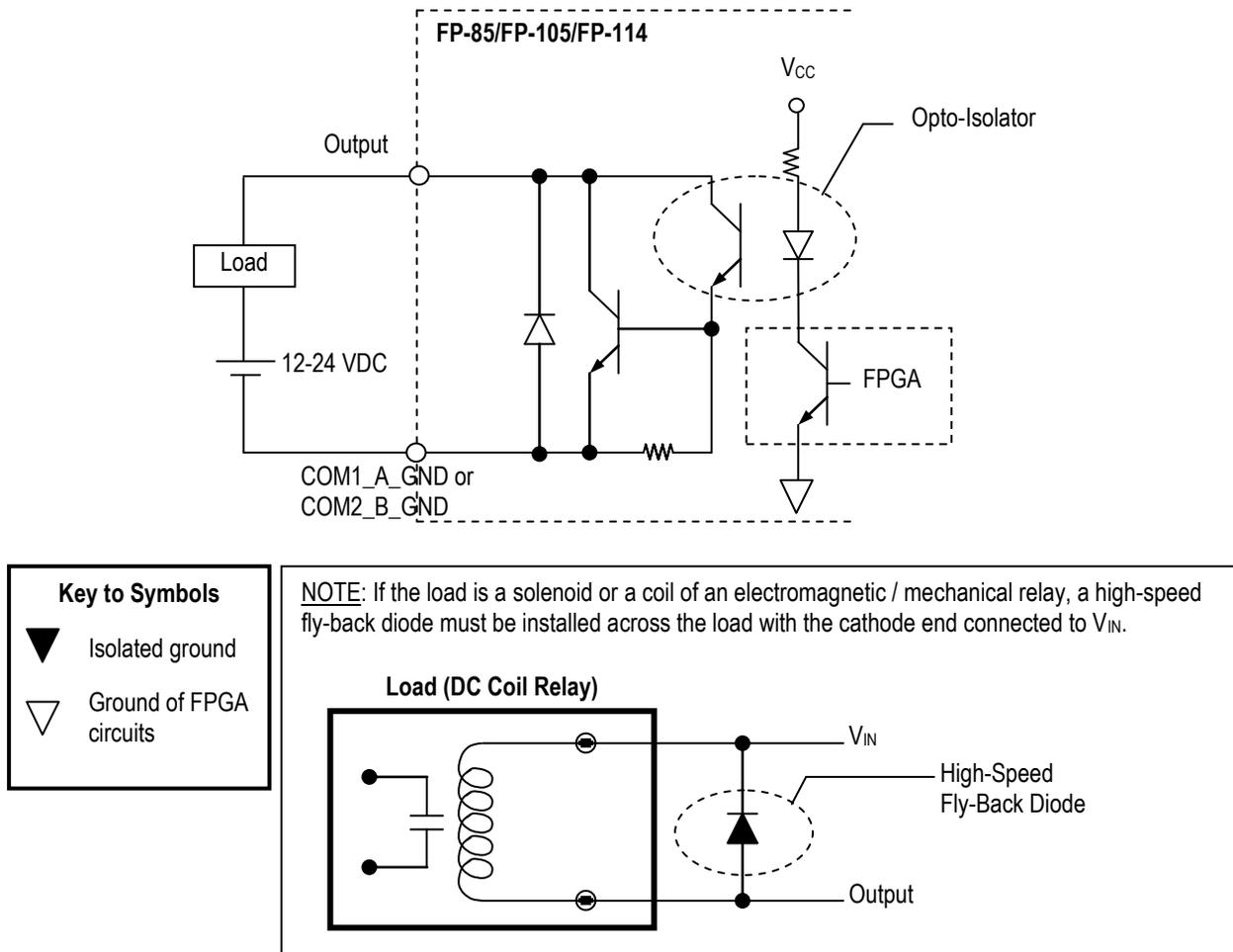
**Figure 1-6: Internal Circuitry and Wiring for OUT00 – OUT15**
