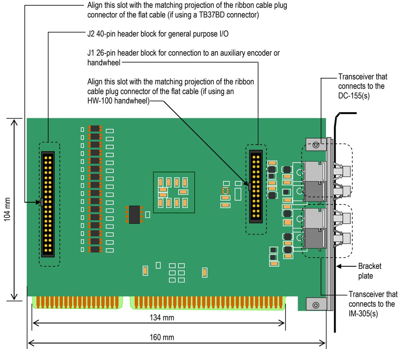
**Figure 1-2: FP-85 VersioBus II Dual-Link Fiber-Optic Adapter Board**
