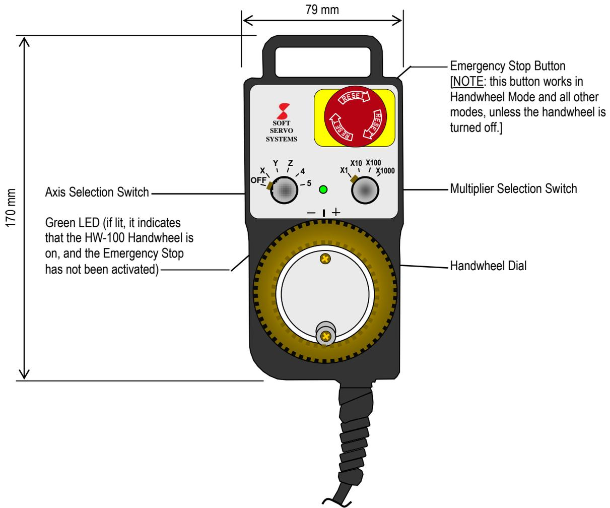
**Figure 6-2: HW-100 Handwheel Schematic Diagram**
