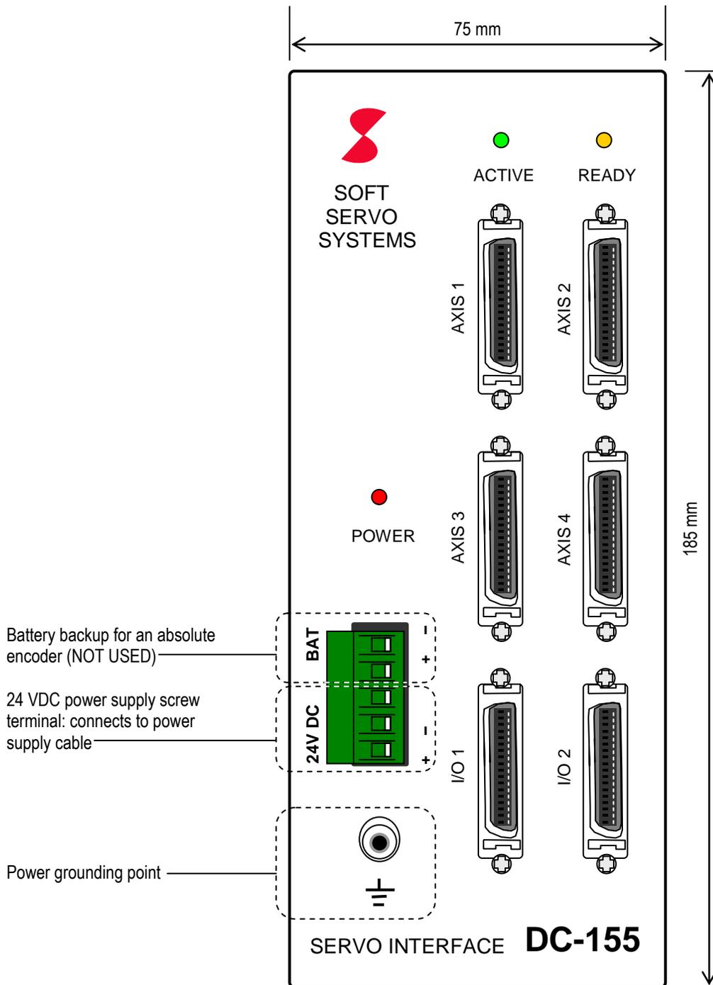
**Figure 2-2: DC-155 VersioBus II Remote Servo Interface Schematic Front Diagram**
