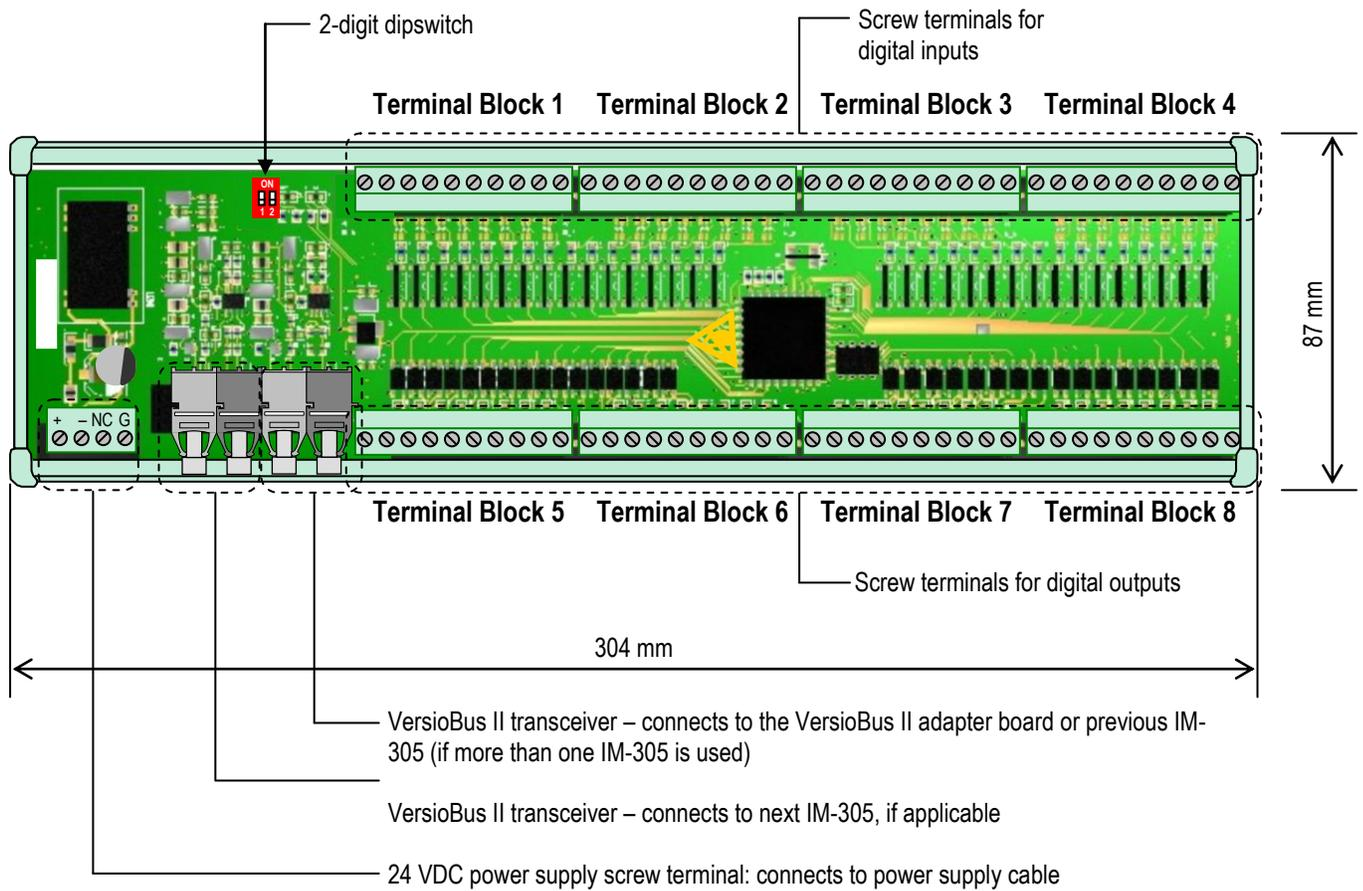
**Figure 3-4: IM-305 VersioBus II General I/O Module Schematic Diagram**
