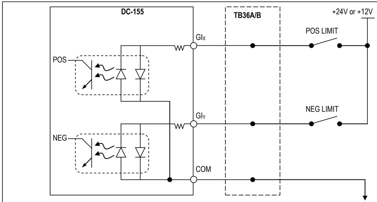
**Figure 8-10: Wiring Example of Normally Closed Limit Switches (Common Ground Connection) Connected to DC-155 General Input**
