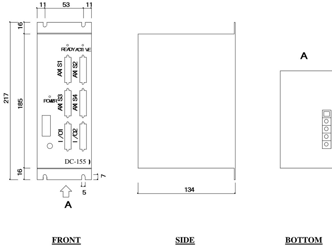
**Figure 2-4: DC-155 Dimensions with Brackets in Millimeters**
