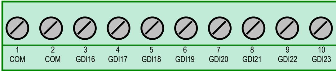
**Figure 3-7: Screw Terminal Numbers for General Digital Inputs (TERMINAL BLOCK 3 – IM-305)**
