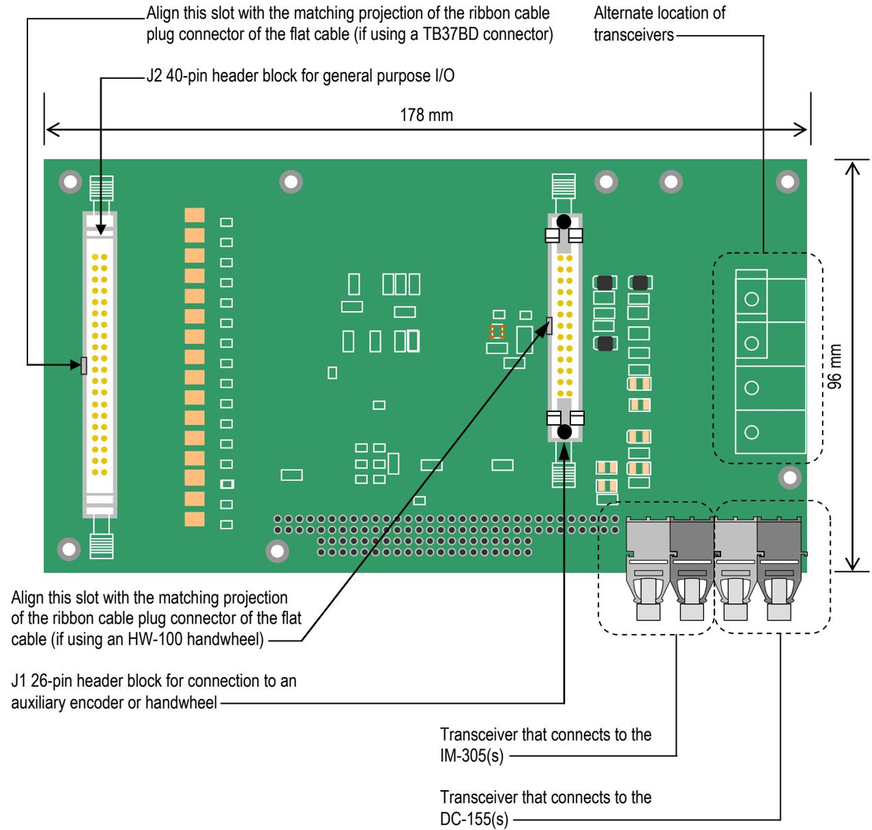
**Figure 1-4: FP-114 VersioBus II Dual-Link Fiber-Optic Adapter Board**
