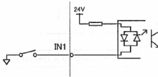
Figure 2-19: Internal Circuitry and Wiring Diagram for DC-125J IN1 Inputs
