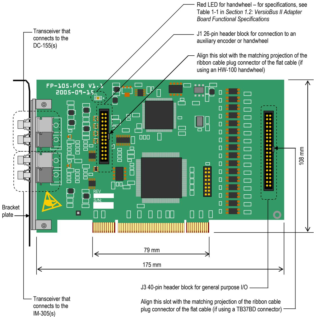
**Figure 1-3: FP-105 VersioBus II Dual-Link Fiber-Optic Adapter Board**
