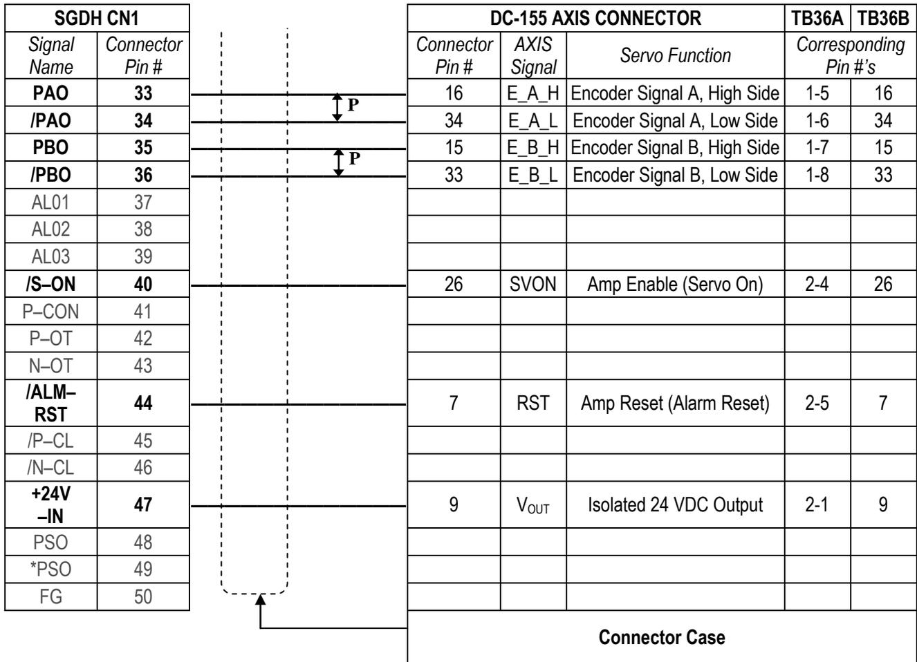
**Table 2-13: Recommended Direct Cable Connections to the YASKAWA Sigma II (SGDH) Servo Drive (2 of 2)**
