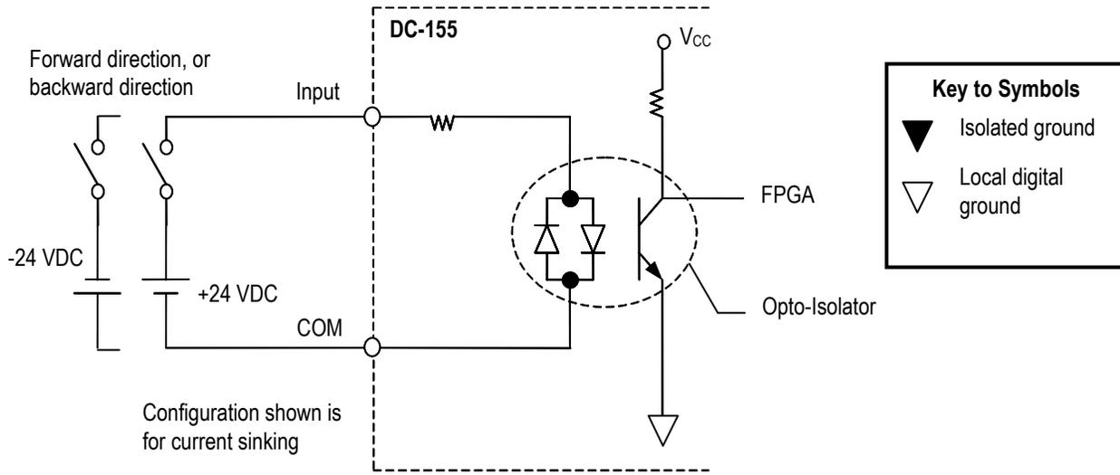
**Figure 2-9: Internal Circuitry and Wiring Diagram for DC-155 General I/O Connector Digital Inputs**
