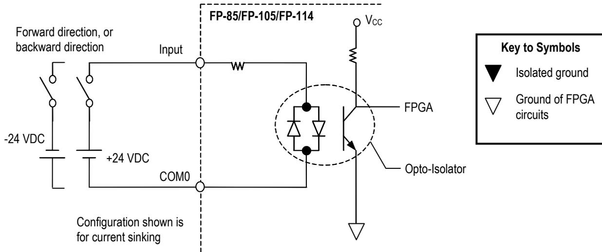
Figure 1-5: Internal Circuitry and Wiring for IN00 – IN15
